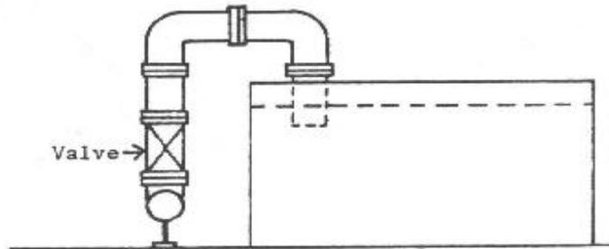
5. A cross connection to a sprinkler system can cause back siphonage when a partial vacuum in the water system draws water from pooled water near a sprinkler head. This type of cross connection led to the "Holy Cross Episode" that was mentioned earlier. Backflow caused by back pressure can occur when the sprinkler head is at a higher elevation than the connection to the potable water system.
