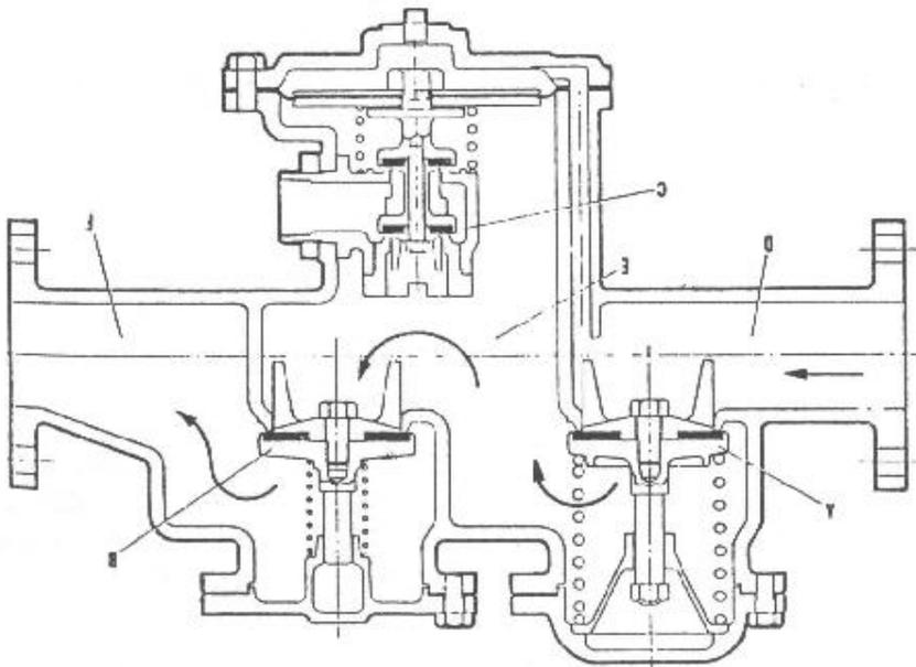
**NOTE: The RPZ above must be accompanied by a valve on both ends to be an approved and testable RPZ assembly.**
