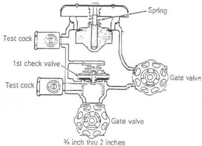
Double checks valve assemblies
