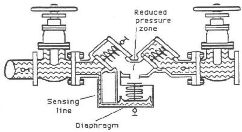
Leaking RPZ. Under special condition during backsiphonage, the relief valve will open, all the water in the reduced pressure zone “dumps”, creating an air gap between check valve #1 and check valve #2.
