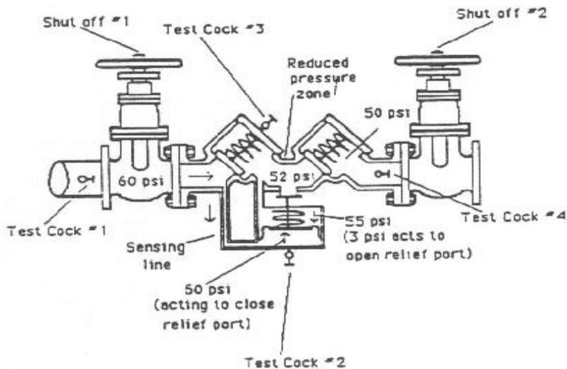
RPZ Under Normal Flow. Assume a supply pressure of 60 psi and a pressure reduction by the first check valve of 8 psi, creating a pressure of 52 psi in the reduced pressure zone. If the relief valve has a 3 psi spring, the pressure working to open the port would be 55 psi (52 psi + 3 psi) and the pressure working to keep the port closed is 60 psi. Thus under normal flow conditions, the relief valve remains open.
