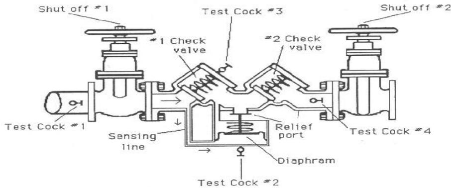
Reduced Pressure Principle Assembly. This backflow preventer is also frequently called a Reduced Pressure Zone Assembly. (RPZ)
