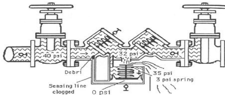
RPZ with Clogged Sensing Line with 0 psi in the Sensing Line. The pressure inside the zone is 32 psi, and the pressure acting to open the relief valve is 35 psi. If the sensing line is clogged and the pressure acting to keep the relief valve closed is 0 psi, the relief valve will open and continue to dump water from the zone until the sensing line is cleared allowing water pressure to the upstream side of the diaphragm.
