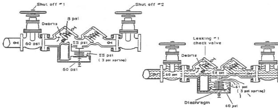
RPZ Failing First Check Valve. Under normal flow conditions, the pressure inside the zone is 52 psi and the pressure acting to open the relief valve is 55 psi. If the first check fails, the pressure inside the zone will increase toward 60 psi. When the pressure inside the zone reaches 58 psi, the total pressure acting to open the diaphragm is 61 psi. This is sufficient pressure to open the relief valve and continuously dump water from the zone.
