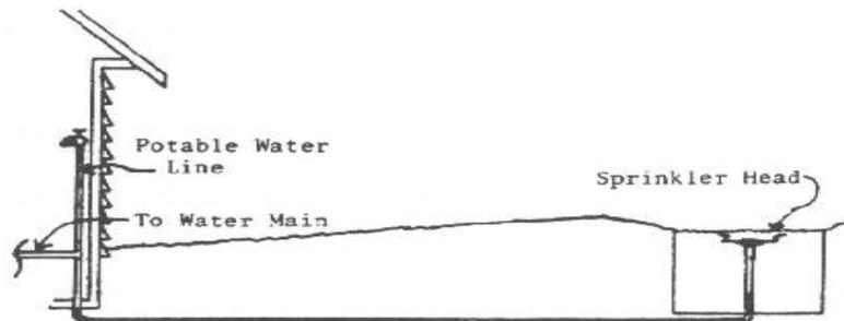
6. A cross connection to a pressurized pipe carrying contaminated water can cause backflow. When the valve is opened, backflow by back pressure can occur if the pressure in the non-potable lines is higher than the positive pressure in the potable system.
