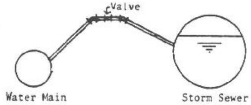
8. When a cross connection to a drain pipe exists, backflow can occur by back siphonage if the valve is left open and there is not enough air gap between the outlet of the cross connection and the drain pipe. A partial vacuum in the potable water line can draw contaminated water from the drain pipe. An example of this would be the drain line from a home water softener.
