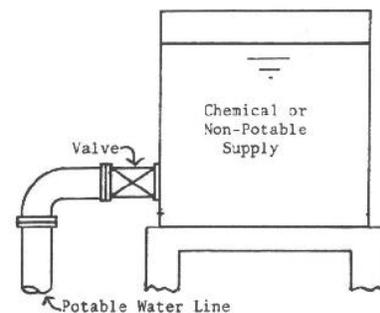
4. A cross connection is created when an open tank is connected to a water line with no air gap. When the valve is opened, back siphonage can occur if a partial vacuum develops in the water system that draws water from the tank into the water system.
