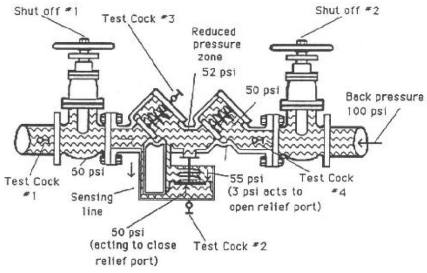
RPZ during Back Pressure Conditions. Assume a supply pressure of 60 psi, a relief valve spring pressure of 3 psi, a spring pressure of 8 psi for the first check valve and back pressure from the downstream side of 100 psi. If the second check valve is working properly the pressure in the reduced pressure zone will not increase.
