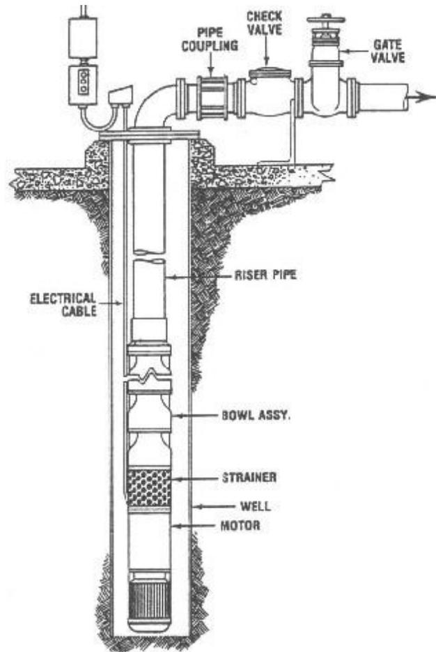
Among other uses, these are used to pump water from at surface source to a treatment plant.
