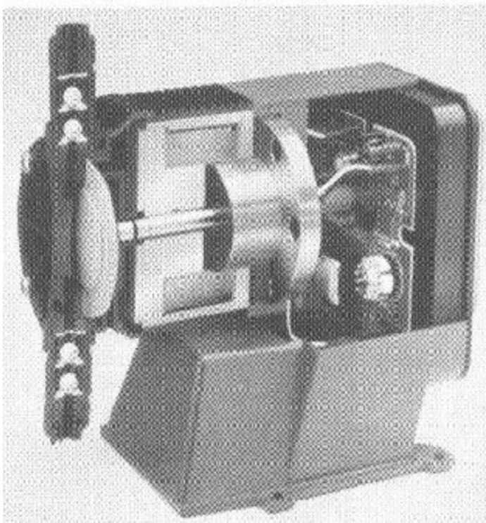
Larger diaphragm pumps may be operated by mechanical means in a fashion similar to the piston pump. The biggest difference is the replacement of the piston with a flexible diaphragm. The diaphragm is attached to a metal rod that is operated by an eccentric cam driven by an electric motor.
